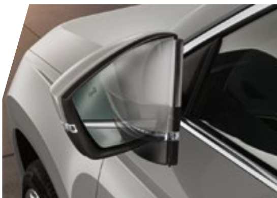
ELECTRICALLY ADJUSTABLE, HEATED AND FOLDABLE DOOR MIRRORS WITH AUTO-DIMMING AND BOARDING SPOTS
