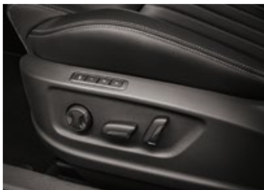
ELECTRICALLY OPERATED DRIVER'S SEAT WITH MEMORY FUNCTION
